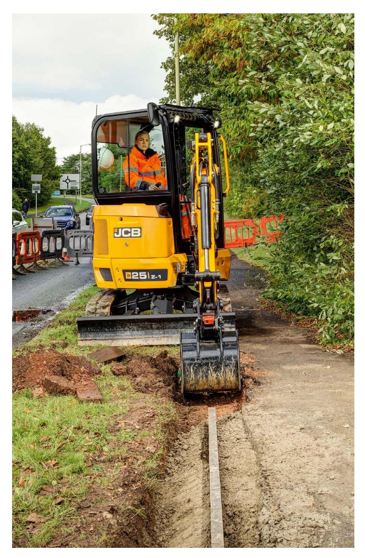
Our robot welded boom and dipper is made from high tensile steel for long life durability.
