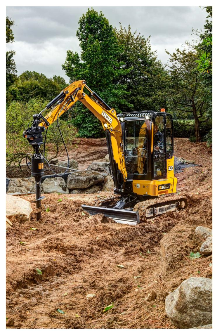
The 25z-1 and 26C-1 have performance enhancements across the hydraulics, tracking, attachments and notably, the new 18.4kW Kohler engine.
