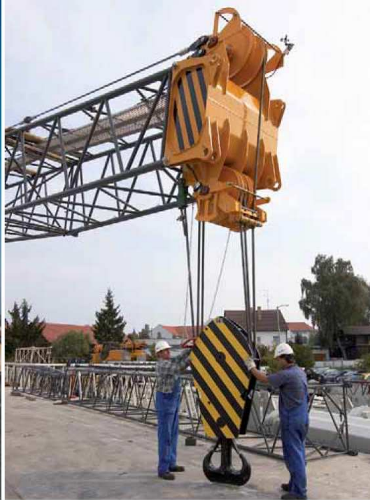
Schwerer Lasthaken am Doppelrollen-Hammerauslegerkopf heavy duty crane hook at the double sheave hammer head
