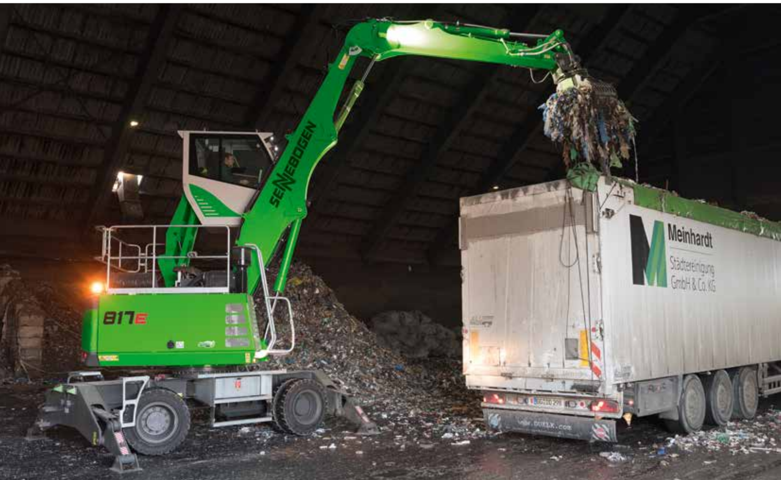
817E - ideal for indoor use/truck loading with compact dimensions, elevating cab and LED-lighting
