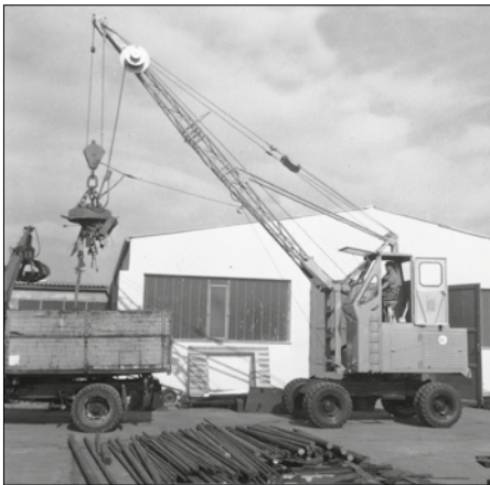
1962: rope-driven S833 with elevated operator cab
