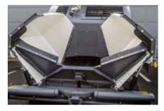
duces material spillage on the push rollers and on the road. It also helps to completely empty the hopper and reduces the need for manual work.
