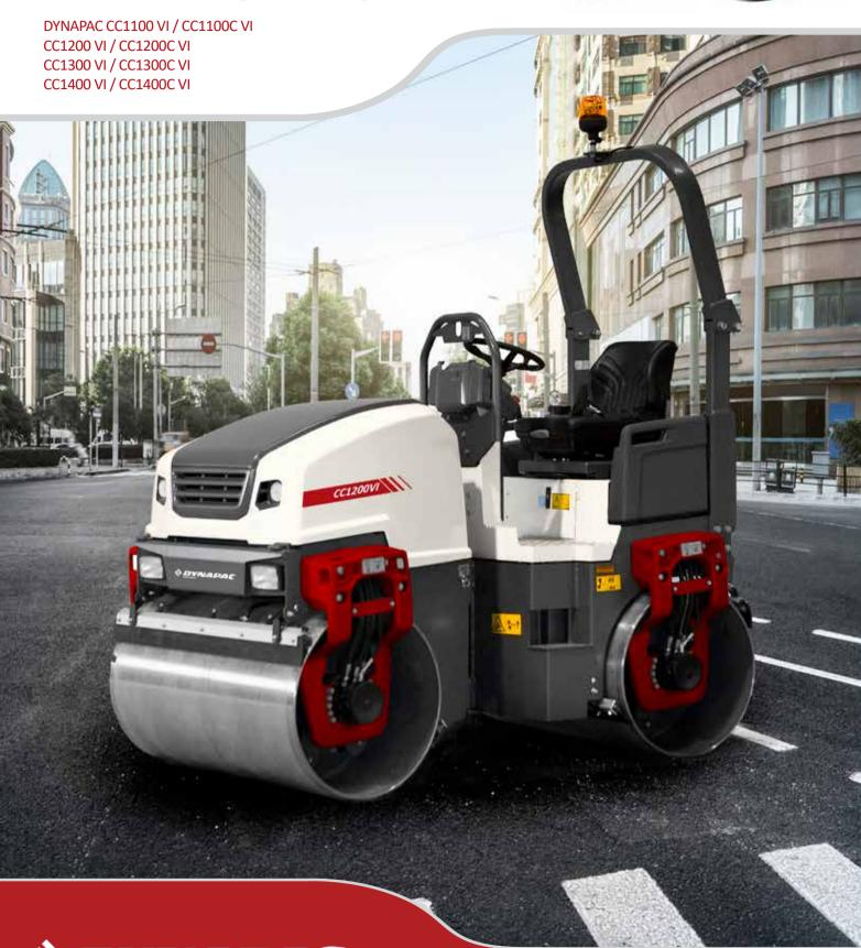
The sixth generation of the Dynapac CC1100/CC1200/CC1300/CC1400 VI small asphalt rollers are designed to meet the construction industry's tough conditions with the operator in mind, resulting in a robust, comfortable and modern machine for best compaction result. The new machine has a unique design with its' cross-mounted engine in combination with an excellent visibility and massive casted forks with flexible lifting/towing/tie down possibilities.
