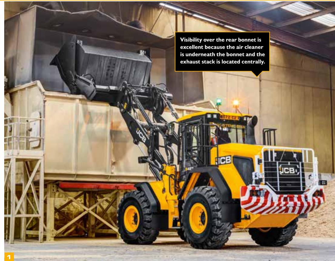
Visibility over the rear bonnet is excellent because the air cleaner is underneath the bonnet and the exhaust stack is located centrally.
