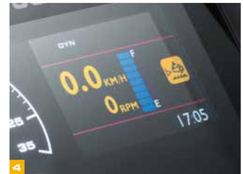
A new auto engine shutdown saves fuel by switching off the engine when the machine is left idling. Idle time can be set by the operator from the cab seat.
