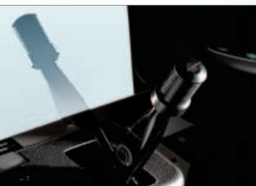
Toggle-type parking brake
