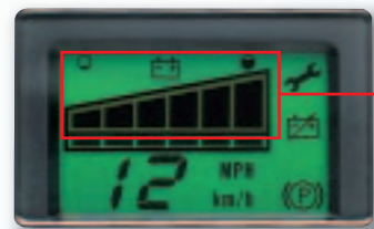
Battery capacity meter
