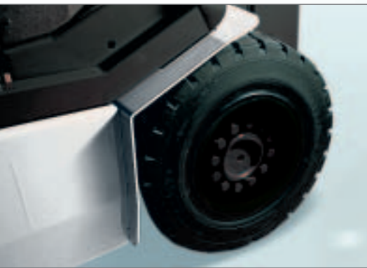
Super-elastic solid tyres (3.0 tonne model shown)
