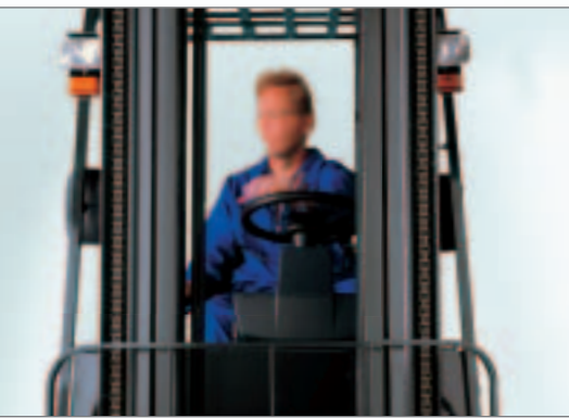
The 2-stage wide view mast with the lift chains mounted on the outside offers superior visibility
