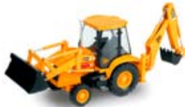
3CX Backhoe Excavator
