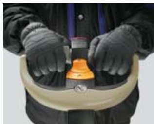
Freezer conditioning for operating temperatures of -30° C
