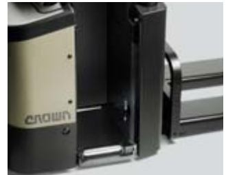
Battery roll-out system
