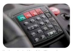
Keyless start, driver identity and access codes ensure no unauthorised operation of your equipment.
