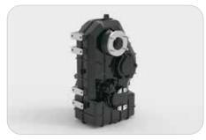
The transfer case inter-axle differential delivers equal torque to each axle when traction is favourable. When conditions deteriorate, the diff-lock automatically engages to deliver torque to the tyres that can best use it.
