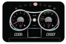
A user friendly 10" colour monitor offers vital operating information, safety warnings, detailed diagnostic readings and dump body function settings.
