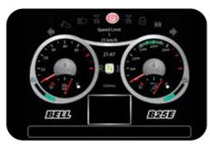
Both operator or site selectable maximum speed control allows the vehicle to automatically decelerate and apply the retarder to prevent onsite speeding.
