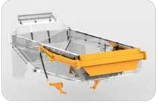
A tailgate is available as an option for better material retention. The tailgate opens as the bin is raised for dumping. Spring steel straps maintain positive seal throughout the haul, ensuring minimal material is lost.
