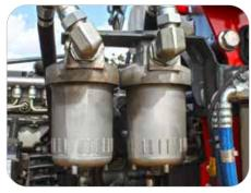
We offer a remote transmission filter option. They make transmission filter replacement a fast and clean task.
