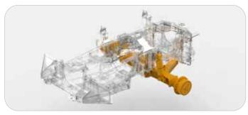
For comfortable productivity, the A-frame suspension system coupled with hydropneumatic suspension struts reduce the lateral vibration often experienced with off-road conditions. A superior suspension seat provides additional isolation for the operator.
