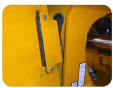
The centralized lube bank places difficult-to-reach grease points within reach.
