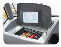
An in-cab load centre simplifies fuse replacement. Fewer relays, connectors and harnesses mean higher reliability.
